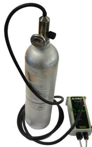
Step [4] Fit the regulator to the 1.6% CO 2 gas bottle
