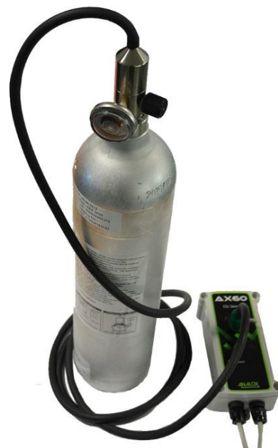
Step [4] Fit the regulator to the O 2 low check gas bottle
